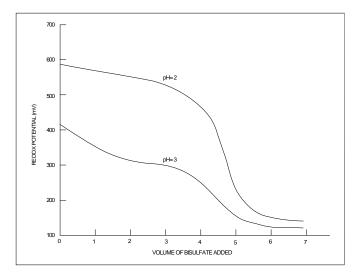
Figure 15-6 Chrome Reduction - Typical Titration Curve
